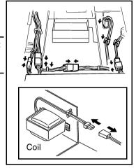
3 Remove three screws and then remove the Power Unit from the machine.(3 screws)
